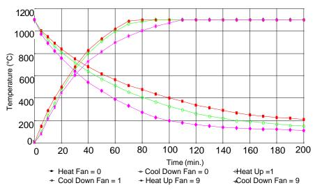
Test Conditions: Nominal line voltage, no load in the muffle only floor tray, full power applied to the muffle for the Heating Curve. The programmable rates are linear and fall below the heating curve and <u>above</u> the cooling curve (door closed) for some selections.
